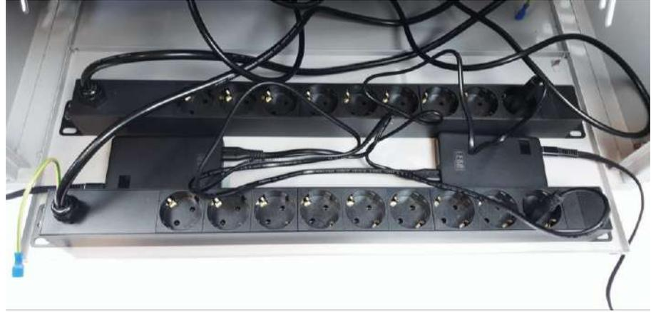
5. When all charging cables are connected use the securing net to lock down the power bricks of the charging cables, to prevent movement during transport. Attach the net by attaching it at the 4 corner points.
