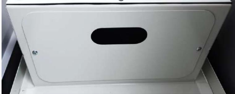
10. Place the electronics compartment door in its original position, reattach the metal clip and lock the door.
